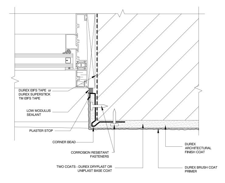
Durabond details are offered to assist in the development of project specific details; principles and variables incorporated in all details are the sole responsibility of the project professional(s).
